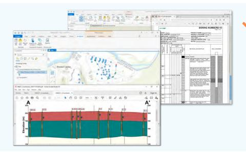
Click locations on a map layer to dynamically generate EQuIS Envirolnsite (EI) graphics, such as boring logs, cross-sections, Piper diagrams, and Stiff diagrams. Graphics are automatically downloaded as PDF files. Envirolnsite license not required.
